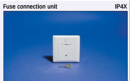
E2030NFSGS WE White 1 gang 250V 13A neon cord outlet cord grip security screw (high) 50Hz Dims: 87x87mm, Fix Ctrs: 60.3mm Mtg.Box: (surface) E238, (flush) BS4662x25mm Material: Polycarbonate Standard: BS 1363 Pt.4:1995
