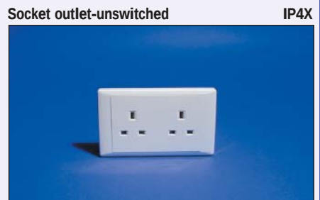
ET2426 WE White 2 gang 250V 13A 50Hz Dims: 148x87mm, Fix Ctrs: 120.6mm Mtg.Box: (surface) E238, (flush) BS4662x25mm Material: Polycarbonate Standard: BS 1363 Pt.2:1995
