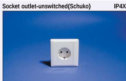
E2426/16 WE White 1 gang 250V 10/16A 2P+E 50Hz Dims: 87x87mm, Fix Ctrs: 60.3mm Mtg.Box: (surface) E238, (flush) BS4662x25mm Material: Polycarbonate Standard: IEC 884-1:1994, VDE 0620
