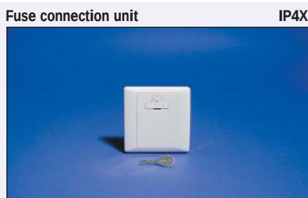
E2030FSGS WE White 1 gang 250V 13A cord outlet cord grip security screw (high) 50Hz Dims: 87x87mm, Fix Ctrs: 60.3mm Mtg.Box: (surface) E238, (flush) BS4662x25mm Material: Polycarbonate Standard: BS 1363 Pt.4:1995
