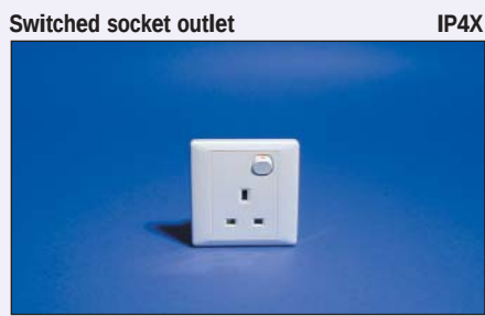
ET2015 WE White 1 gang SP 250V 13A 50Hz Dims: 87x87mm, Fix Ctrs: 60.3mm Mtg.Box: (surface) E238, (flush) BS4662x25mm Material: Polycarbonate Standard: BS 1363 Pt.2:1995
