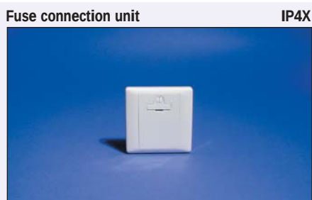
E2030FSGMS WE White 1 gang 250V 13A cord outlet cord grip security screw (medium) 50Hz Dims: 87x87mm, Fix Ctrs: 60.3mm Mtg.Box: (surface) E238, (flush) BS4662x25mm Material: Polycarbonate Standard: BS 1363 Pt.4:1995
