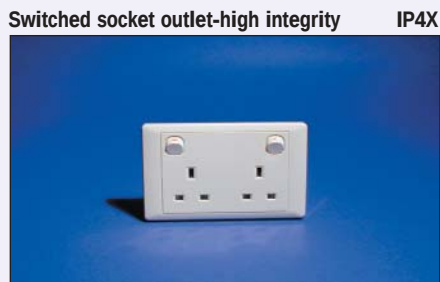
ET2025D WE White 2 gang DP 250V 13A 2 Earth terminals 50Hz Dims: 148x87mm, Fix Ctrs: 120.6mm Mtg.Box: (surface) E238, (flush) BS4662x25mm Material: Polycarbonate Standard: BS 1363 Pt.2:1995
