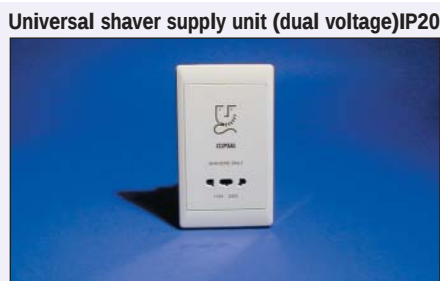
ET2727 WE White 240/110V 20VA 50Hz Dims: 147x87x56mm, Fix Ctrs: 120.6mm Mtg.Box: (surface) E238D, (flush) BS 4662x45mm Material: Polycarbonate Standard: BS 3535 Pt.1:1990, BS EN 60742:1996
