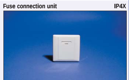
E2030FSG WE White 1 gang 250V 13A cord outlet cord grip 50Hz Dims: 87x87mm, Fix Ctrs: 60.3mm Mtg.Box: (surface) E238, (flush) BS4662x25mm Material: Polycarbonate Standard: BS 1363 Pt.4:1995
