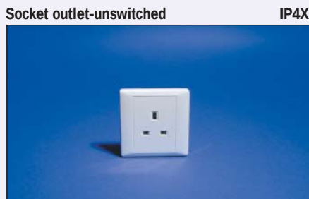
E2426 WE White 1 gang 250V 13A 50Hz Dims: 87x87mm, Fix Ctrs: 60.3mm Mtg.Box: (surface) E238, (flush) BS4662x25mm Material: Polycarbonate Standard: BS 1363 Pt.2:1995
