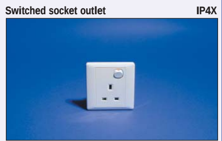
E2015D WE White 1 gang DP 250V 13A 50Hz Dims: 87x87mm, Fix Ctrs: 60.3mm Mtg.Box: (surface) E238, (flush) BS4662x25mm Material: Polycarbonate Standard: BS 1363 Pt.2:1995
